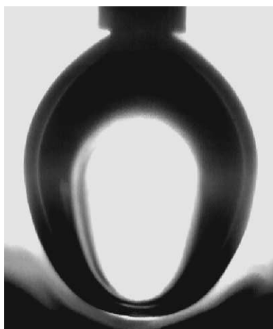
Fig. 7. Water drop in corn germ oil containing CO 2 , 200 MPa, 293 K. The turbid front at the bottom influences the drop shape.
